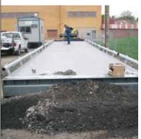
Installation can be as easy as setting the premium portable scale on solid, level ground and forming an earthen ramp at each end. The basic portability option requires field assembly. Bolt the frame components together, set the scale modules in place, and provide ramps.
