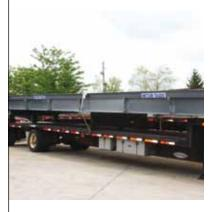
The premium portable design can be moved in one piece. Simply lift the scale and its attached frame onto a flat-bed trailer for transport. The basic portability option requires removing the scale modules and dismantling the frame before loading the components onto a trailer to be moved.
